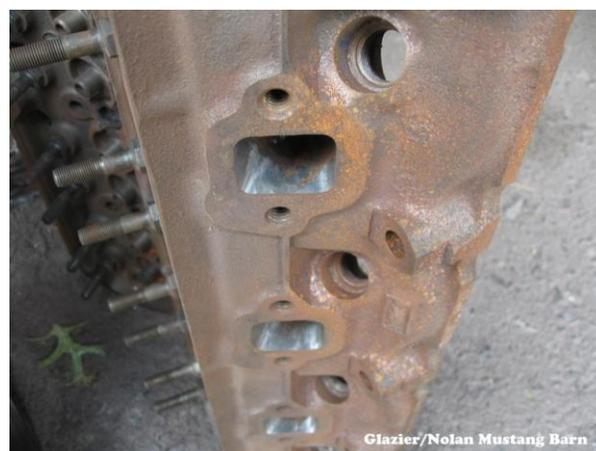
This is a 289 High Performance head which has already been ported. The opening itself had been very restrictive, but it is not necessary to go deeply into the port, usually only 1/2" – 3/4" or so inward from the gasket surface. The improvement is astonishing.
