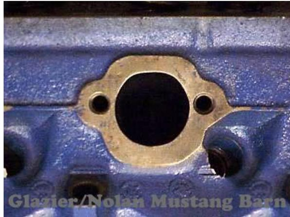
There is a lot to work with, though. Crane used to offer "Fireball" heads (shown above), which started out as over-the-counter Ford K code (and later J code) replacement heads, and Crane would dramatically open the exhaust ports, far beyond what I would recommend, especially since they then required special "Fireball" headers.
